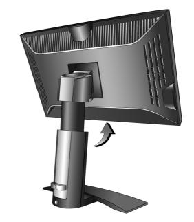
Rotate the monitor 90 degrees counter-clockwise (from the rear side) as illustrated.
